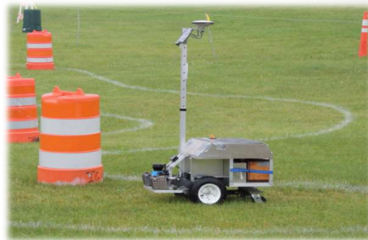
AGV attempting to avoid an obstacle
